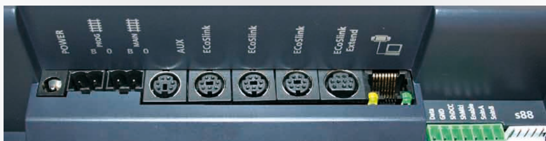
ESUslot expansion port for ECoSControl Radio Power-In jack Programming track connection Main track connection ECoSlink systems input socket ECoSlink systems input socket ECoSlink systems input socket ECoSlink systems expansion socket Ethernet connection DCC Booster out ECoSniffer input s88 input
