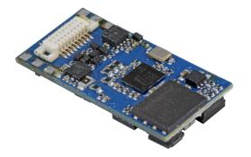
The LokSound 5 micro is a "little wonder": With only 21mmx10mm footprint, it is by far one of the smallest LokSound decoders we've ever built. This is perfect for N scale, but can also be used in small H0 locos. LokSound 5 micro decoders always have a Next18 interface and are offered with adapter plugs for all common interfaces.
