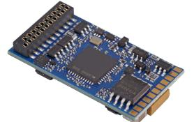
The LokSound 5 is the most important member of the LokSound family. Due to the combination of digital decoder and sound module on a printed circuit board, the decoder is only 30mm x15.5mm and can be installed in almost any locomotives of in H0, S, or 0 gauges if the max amperage draw is under 1.5 amp.
