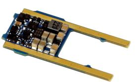
The LokSound 5 micro DCC Direct Kato Japan has been specially developed for installation in Kato-branded N gauge locomotives: in many European and Japanese locomotives of this manufacturer, the ser decoder can be installed directly below the engine instead of the analog board installed as standard. Finally, these models can also be easily retrofitted with a LokSound decoder.
