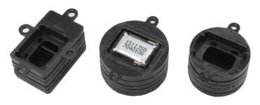
With our new modular speaker baffle set suitable for a single miniature speaker you can easily assemble your tailormade speaker baffle for two miniature speakers. Both – diameter and height – can be individually adapted to suit your needs. Even with one speaker the audio pressure is considerably better than with one circular speaker intended for these dimensions.
