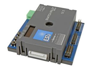
SwitchPilot 3 servo decoders are optimized for stationary use on your system and can control up to eight RC servo drives. In order to facilitate the rather cumbersome configuration of magnetic article decoders, the SwitchPilot 3 Servo has an innovative operating concept consisting of a 4-line, illuminated OLED display and three input buttons.
