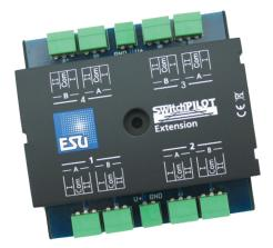
If required, SwitchPilots and SwitchPilot Servos can be augmented with the SwitchPilot Extension Module: Plugged in at the side of the Switch-Pilot, it offers four relay-driven outputs, used for switching potentialfree loads, or for polarizing the frog; the ideal supplement for tricky circuitry.
