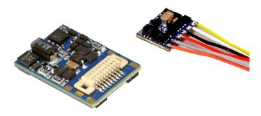
The LokPilot 5 micro DCC is the "twin" of the LokPilot 5 micro. With just 8.0mm x 7.0mm and a thickness of only 2.4mm (on the capacitor: 2.9mm), just so small that it can also be accommodated in very small locomotives of nominal sizes Z, N or TT, it is a pure DCC Decoder. This lack of flexibility is rewarded with a lower price.
