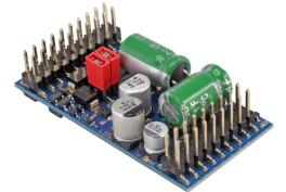
The LokSound 5 L finds its place in O Scale between the LokSound 5 and the LokSound 5 XL. With dimensions of just 51mm x 25.5mm, it is not only recommended for size 0 scale locomotives, but also for all other models where a LokSound 5 XL does not fit or is required.
