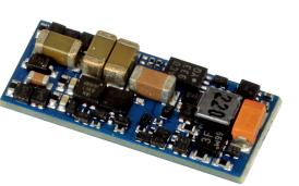
With the LokSound 5 Nano DCC, ESU has succeeded in developing an even smaller LokSound decoder: With only 19.6 mm x 8.5 mm x 3.2 mm, it is the smallest LokSound decoder we have ever built. Thus, it should really be used in all vehicles of nominal sizes N and TT.
