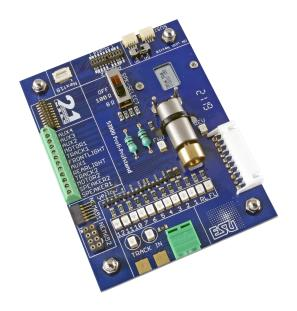
Maybe you know the situation: In front of you there is a digital decoder on the workbench, and before you undertake its complicated installation into the loco, you would like to know if the decoder works as advertised. But, how do you test it? The Decoder Tester helps you: It's designed for testing decoders before these are installed into a loco. The Decoder Tester is simply hooked up to your digital command station, or the LokProgrammer. It even works well with non ESU decoders!
