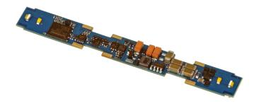
The LokSound 5 micro DCC Direct has been specially developed for installation in N gauge locomotives of the Atlas and Intermountain brands: it can be inserted directly instead of the analog board installed there as standard. However, the decoder can also be used for similar models from other manufacturers at your own discretion.
