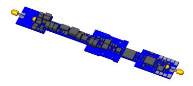
The LokSound 5 micro DCC Direct Kato USA has been specially developed for installation in N gauge locomotives of the Kato USA brand: Most diesel locomotives of this manufacturer are installed in the American model of these decoders instead of the analog board installed as standard. Finally, these models can also be easily retrofitted with a LokSound decoder.
