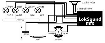
$\textbf{Figure 3}: \ \ \text{Wiring of engines with DC motors and functions with the common pole connected to the chassis}$
