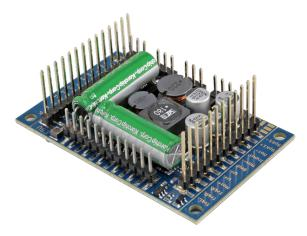
The LokSound 5 XL decoder is an extremely powerful decoder! It must be as it is intended for use in your garden railway or 1/G gauge locomotives. Its integrated, power-adapted PowerPack ensures safe operation even on dirty tracks.
