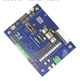
Maybe you know the situation: In front of you there is a digital decoder on the workbench, and before you undertake its complicated installation into the loco, you would like to know if the decoder works as advertised. But, how do you test it? The Decoder Tester helps you: It's designed for testing decoders before these are installed into a loco. The Decoder Tester is simply hooked up to your digital command station, or the LokProgrammer. It even works well with non ESU decoders!
