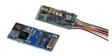
With the LokSound 5 Nano DCC, ESU has succeeded in developing an even smaller LokSound decoder: With only 19.6 mm x 8.5 mm x 3.2 mm, it is the smallest LokSound decoder we have ever built. Thus, it should really be used in all vehicles of nominal sizes N and TT.
