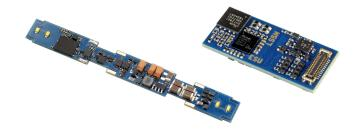
The LokPilot 5 micro DCC DCC Direct and the LokPilot 5 nano DCC are the "little brothers" of the LokSound 5 micro DCC Direct and the LokSound 5 nano DCC. These non-sound Decoders share the same dimensions and functions with the LokSound decoders, but without sound.
