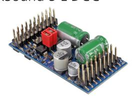
The LokSound 5 L finds its place in O Scale between the LokSound 5 and the LokSound 5 XL. With dimensions of just 51mm x 25.5mm, it is not only recommended for size 0 scale locomotives, but also for all other models where a LokSound 5 XL does not fit or is required.
