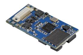
The LokSound 5 micro is a "little wonder": With only 21mmx10mm footprint, it is by far one of the smallest LokSound decoders we've ever built. This is perfect for N scale, but can also be used in small H0 locos. LokSound 5 micro decoders always have a Next18 interface and are offered with adapter plugs for all common interfaces.
