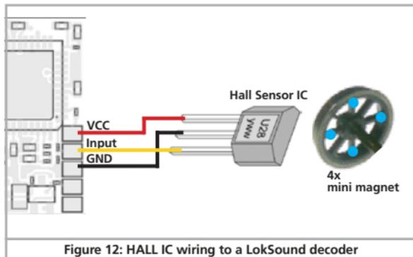
Figure 12: HALL IC wiring to a LokSound decoder
