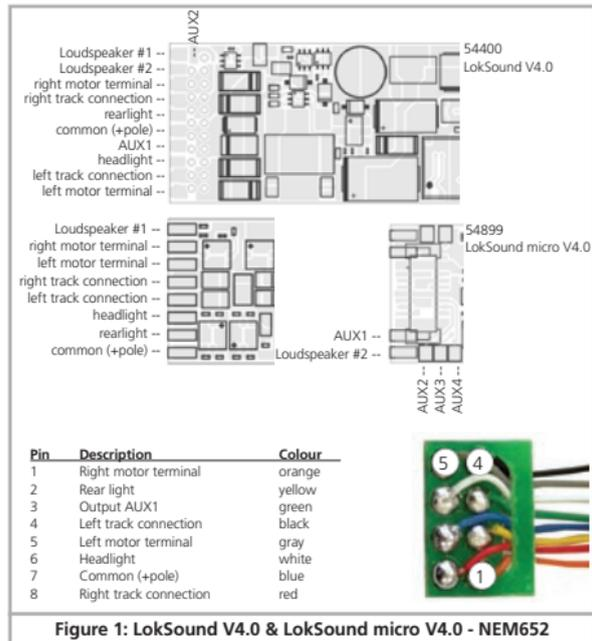
Figure 1: LokSound V4.0 & LokSound micro V4.0 - NEM652
