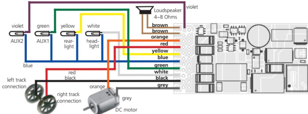
Figure 4: Wiring Diagram for LokSound V4.0 (wiring example)
