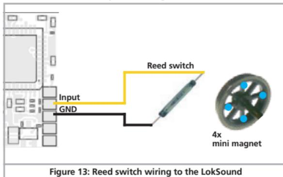
Figure 13: Reed switch wiring to the LokSound
