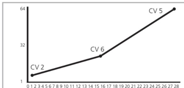
Figure 15: Speed settings using CV 2, 6, 5
