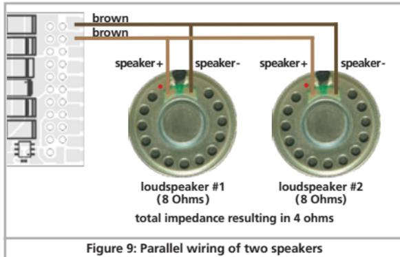
Figure 9: Parallel wiring of two speakers
